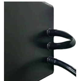
Two Unused outlets connected with tubing
